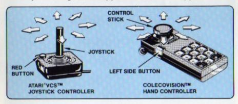
The **left** side button on your standard ColecoVision™ hand controller functions just like the red button on the Atari® VCS™ joystick controller.
