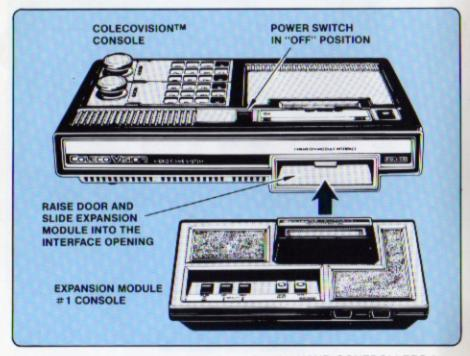
Now that the units are connected, unplug the HAND CONTROLLERS from ColecoVision™ Console and plug them into the sockets in front of the Expansion Module as shown. NOTE: Either ColecoVision™ or Atari®VCS™ compatible controllers will fit into the sockets of your Expansion Module.
